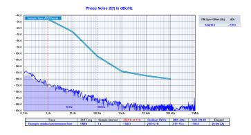
53100A phase noise test software is shipped along with the product. It allows a user to set up various measurement configurations/speeds, toggle display settings, import/export data, run scripts, set up mask lines and more.
